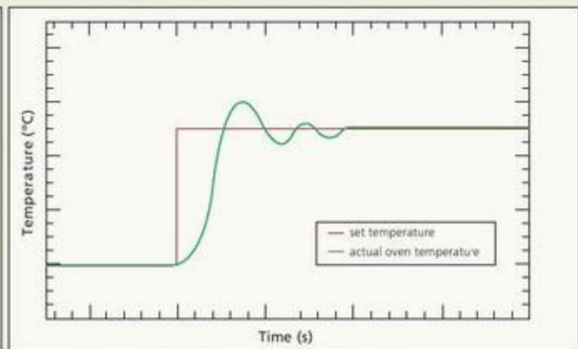
Figure 3: Oven temperature change for a set temperature increase – variable heater with proportional (P) controller
