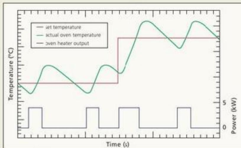
Figure 2: Oven temperature change for a set temperature increase – on-off heater system
