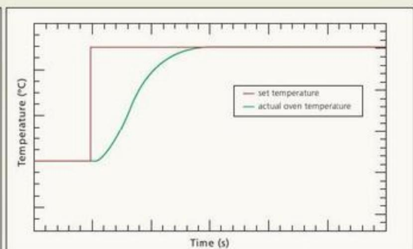
Figure 5: Oven temperature change for a set temperature increase – variable heater with proportional, integral and derivative (PID) controller
