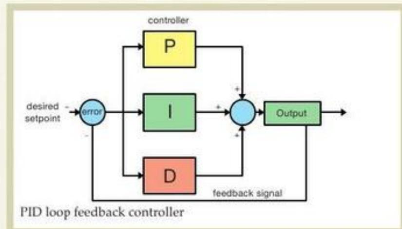
only supply heat if the oven temperature and set temperature are different. This is known as offset or droop.
