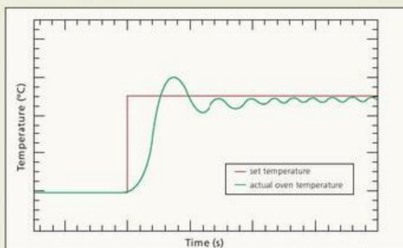
Figure 4: Oven temperature change for a set temperature increase – variable heater with proportional and integral (PI) controller
