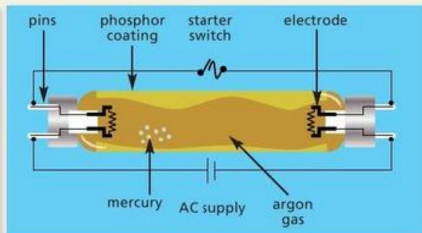
Figure 2: Turn on lamp → current flows to electrodes creates voltage difference → free electrons move through gas → mercury changes from liquid to gas → electrons collide with gaseous mercury atoms → atoms emit ultraviolet light photons → photons hit phosphor atoms → phosphor releases white light
