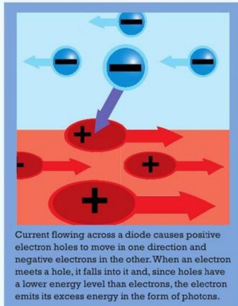
Current flowing across a diode causes positive electron holes to move in one direction and negative electrons in the other. When an electron meets a hole, it falls into it and, since holes have a lower energy level than electrons, the electron emits its excess energy in the form of photons.
